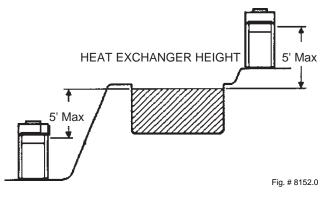
**NOTE:** If heater is installed outside of the limits shown, a flow switch must be used in place of the pressure switch when mounted and wired adjacent to the heater.
